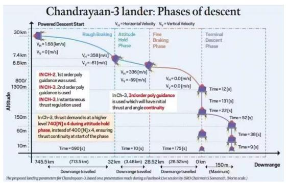
The final critical manoeuvre is the fine braking phase. During this phase, the lander will be aligned vertically and will hover at a height of **800 to 1,300 meters** above the landing site. The lander will then use its thrusters to make small adjustments to its position in order to land safely.
