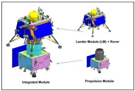
**Propulsion Module:** The propulsion module is responsible for carrying the lander and rover configuration to the lunar orbit of 100 kilometers. It is a box-like structure with a large solar panel and an intermodular adapter cone that acts as a mounting structure for the lander. Additionally, it carries the SHAPE payload, which studies spectral and polarimetric measurements of Earth from the lunar orbit.
